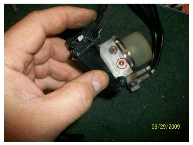
I now used a Dremel Tool to clean up the hydraulic fittings. This is not just a anal move. Hydraulics REQUIRE cleanliness...
