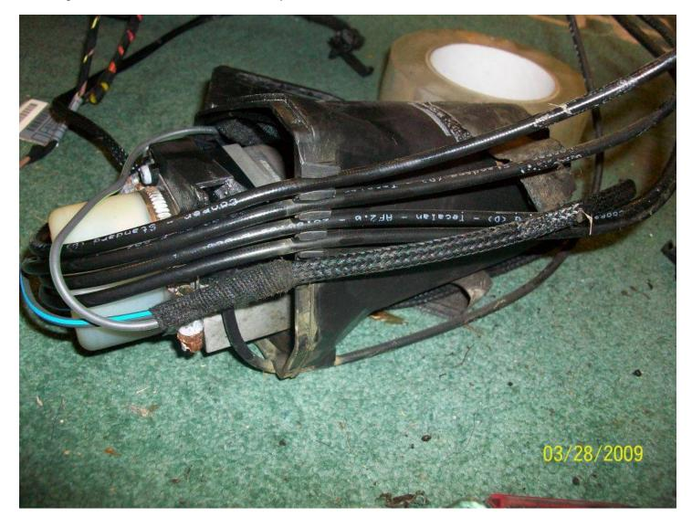
As extra insurance, before I pulled the motor out, I labeled the hydraulic lines. 3,4,5,6. and then after the motor was out of the housing, labeled the old housing the same way. Just to be sure.
