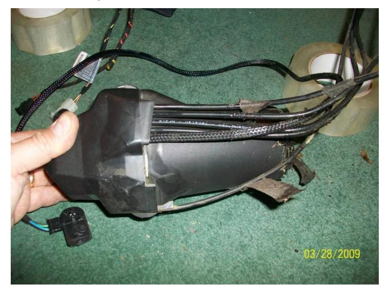
Housing cover removed. You can already see the corrosion.
