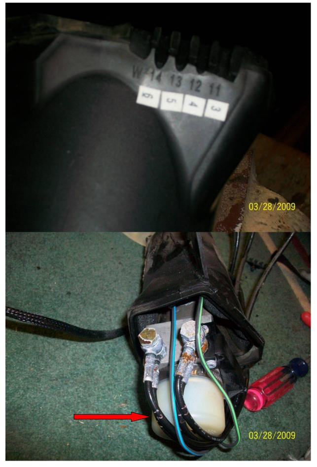
Remove the electrical connectors and clean them up. Use Q-Tips, Pipe Cleaners, whatever. I removed the boots and cleaned them up also. Carefully note which way the wires connect and what terminals they go on. If you put them on backward, the top will operate in reverse and you will have to remove the soft top and redo.
