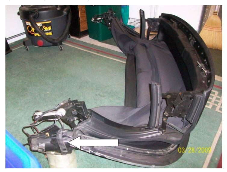
Remove the mount from the top frame and note (Take a picture) of the wiring and hydraulic line placement.
