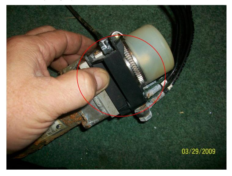
The Bowden Cable Assembly. Looking at the motor, the brass button on the bottom is the actual hydraulic by-pass plunger. This shifts the internal spool allowing oil to flow freely, without the motor driving it.
