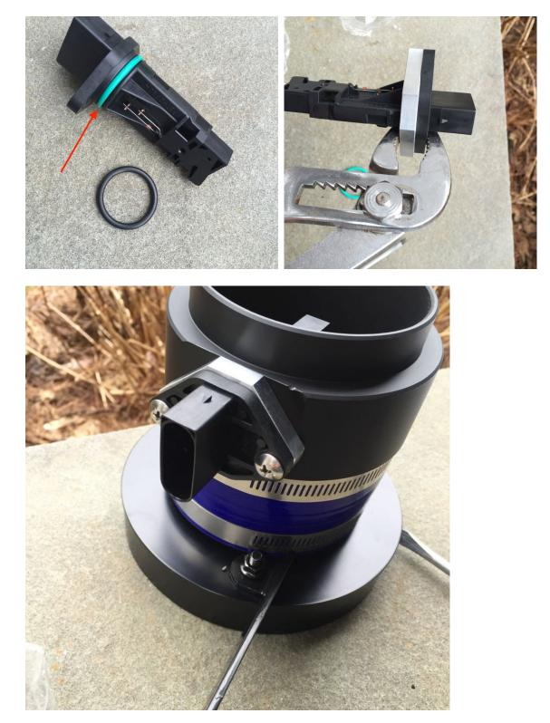
Attaching the support bracket requires holding a nut and washer under the small metal lip where the airbox was previously attached. This requires some finesse. A towel can be placed in this area to trap the nut and washer if they should fall. The bracket is held in place with bolt A. The carbon fiber intake is joined to the metal adapters by high quality band clamps. The intake should be placed roughly into position <u>before</u> mounting the support bracket.
