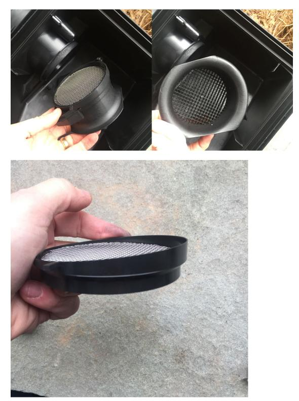
Remove plastic tube and push out the wire mesh insert.
