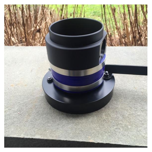
Replace the existing green o-ring on the MAF sensor with the thicker o-ring supplied. It may require some extra force to fully seat the MAF sensor into the aluminum sensor spacer before screwing it into the MAF tube.
