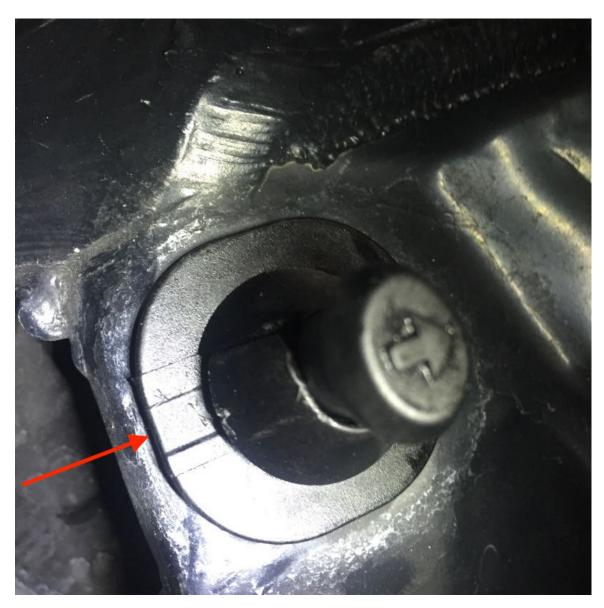
Note the small slot on the connector base. Using a small flat blade screwdriver in this slot, pry up the connector.
