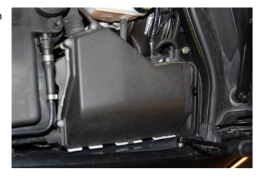
**Step 3:** Unbolt the 4 bolts holding the cover using a T20 torx driver and lift the cover aside.
