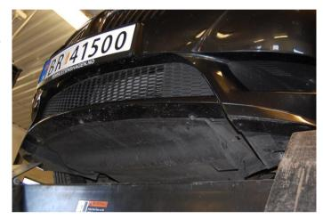
**Step 20:** Push the centre of the clip holding the inner fenders to the bumper.
