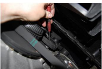
**Step 36:** Remove the belt using a 8mm hexagon tool on the centre bolt for the tensioner pulley. Push the tensioner pulley clockwise to release the tension.
