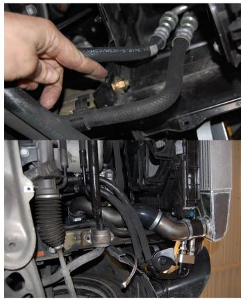
**Step 53:** Secure the power steering hoses using supplied tie wraps. Make sure it does not conflict with the belt.
