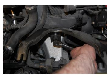
**Step 16:** Remove the oil drain hose from the side of the oil pan.
