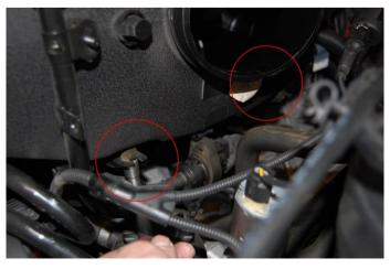
**Step 13:** Loosen the 6 clips holding the manifold to the throttle bodies.
