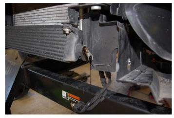
**Step 28:** Unbolt the 4 bolts holding the front oil cooler element using a 5mm hexagon tool and a T50 torx socket and lift the oil cooler aside.
