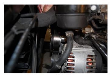
**Step 41:** Unbolt the two bolts holding the alternator using a 16mm socket wrench.
