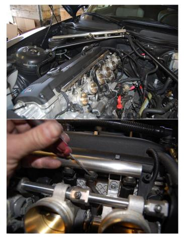
**Step 56:** Remove the clip holding the fuel rail to the fuel line.
