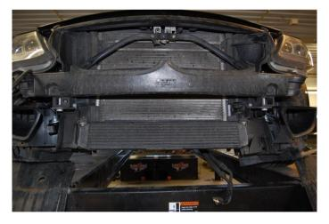
**Step 29:** Remove the front part of the inner fenders on each side. **ONLY ON VT2-500**
