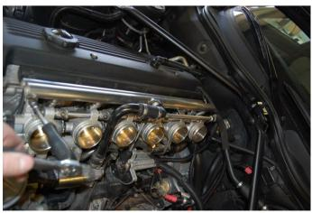
**Step 55:** Unclip the idle control valve hose from the vacuum rail and lift the rail aside.
