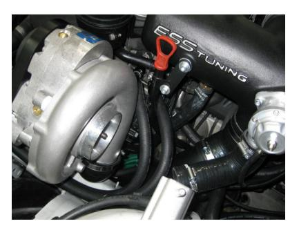
**Step 33:** Install the intercooler. Use the standard torx bolt that previously was holding the stock oil cooler. Adjust the cooler to center position. Do not secure the bolt fully at this moment. **ONLY ON VT2-500**
