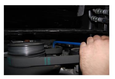
**Step 37:** Unclip the clamp holding the power steering hose from the tank to the power steering pump on the pump side and drain the fluid.
