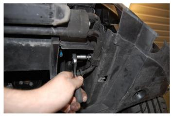
**Step 26:** Unbolt all the bolts holding the front part of the inner fender on each side. **ONLY ON VT2-500**
