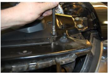
**Step 73:** Locate the two plastic clips holding the air duct and remove them. Pull the air duct out.
