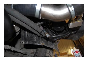
**Step 84:** Cut the plastic inner fender to make room for the pressure tubes and oil lines for the oil cooler and reinstall them using standard bolts. **ONLY ON VT2-500**
