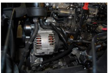
**Step 40:** Remove the plastic cover on the outside of the upper idler pulley (top alternator bolt) using a flathead screwdriver.
