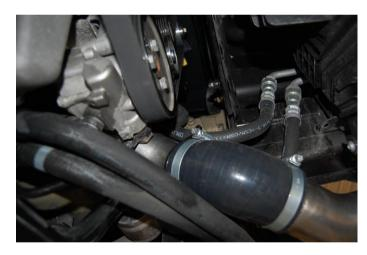
**Step 54:** Unbolt the two M6 bolts holding the fuel rail using a 10mm socket.
