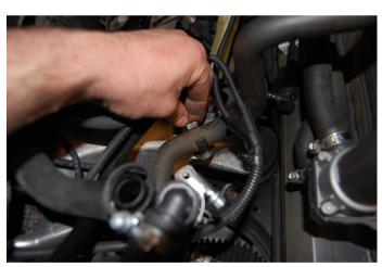
**Step 62:** Remove the plastic quick connector located on the idle control valve hose.
