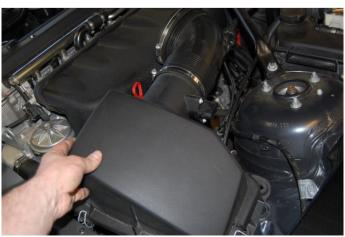
**Step 9:** Unclip the crankcase ventilation breather hose from the inlet manifold.
