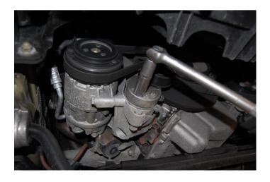
**Step 51:** Remove the bracket holding the power steering hoses using a 13 mm socket. **ONLY ON VT2-500**
