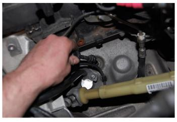
**Step 17:** Plug the hole using the supplied ESS plug.
