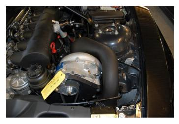
**Step 77:** Cut the plastic hose loose from quick connector on top of the valve cover.
