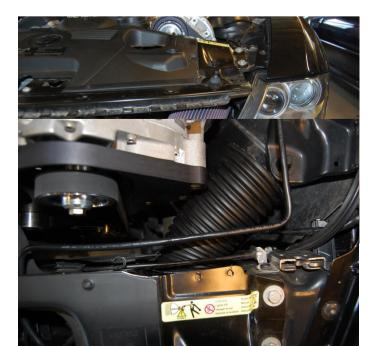
**Step 76:** Install the supplied ESS plastic inlet tube. Adjust the clearance towards the inner fender and secure the clamps.
