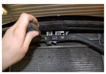
**Step 32:** Installed supplied ESS oil cooler and lines using the stock bolts. Connect the hoses to the oil adapter. Route the hoses and adapter in the way shown in the picture and secure the bolts. **ONLY ON VT2-500**
