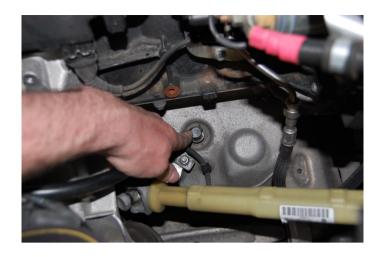
**Step 18:** Unbolt the 7bolts holding the front bumper on the top using a T30 Torx driver.
