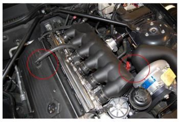
**Step 78:** Install the 38mm 90 degree hose from the bypass valve to the inlet on the plastic inlet tube. Secure the clamps.
