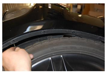
**Step 21:** Push in and back to release the bumper on each side.
