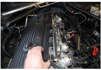
**Step 58:** Remove the lower o ring from the stock injector and install it on the new supplied ESS injector.
