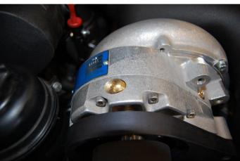
**Step 82:** Check the oil level in the supercharger using the dipstick tube. There is most likely to much oil in the charger. Adjust the level by draining out of the drain hose until the oil level is at max on the dipstick.
