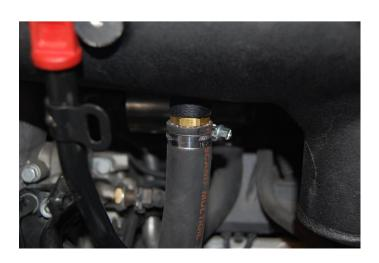
**Step 68:** Install the bracket for the dipstick tube using supplied bolts.
