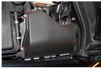
**Step 4:** Remove the ECU and send it to ESS for reprogramming.
