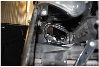
**Step 75:** Install the air filter with 3.5 inch flex hose through the hole. It is very tight to get the air filter into position.
