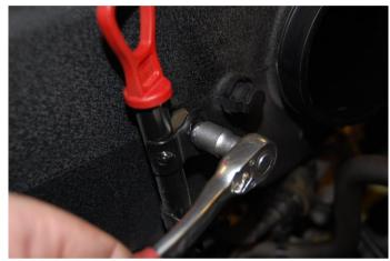
**Step 11:** Unclip the idle control valve hose from the underside of the manifold.
