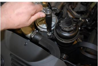
**Step 47:** Install the second idler pulley in the threaded hole at the bottom of the bracket. Remember the spacer between the bracket and the pulley. Secure the bolt using a 8mm hexagon tool.
