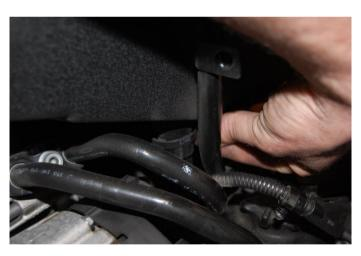
**Step 12:** Unbolt the two M6 bolts holding the manifold to the steel bracket on the underside of the manifold using a 10mm socket.
