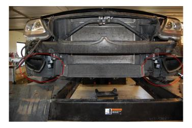
**Step 27:** Unbolt the bolt holding the oil lines to the front cooler using a 6 mm hexagon tool and drain the oil. **ONLY ON VT2-500**
