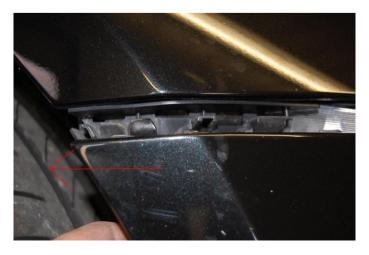
**Step 22:** Lift the bumper a little away from the car and block off the hose for the front headlight washers.
