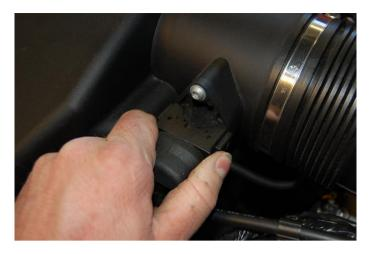
**Step 6:** Disconnect the plastic tube coming from the brake booster line going into the inlet tube going from the mass air sensor to the inlet.
