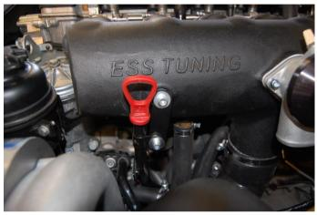
**Step 69:** Pull the rubber cap from the vacuum outlet on the back of the vacuum rail and connect the vacuum hose from the bypass valve. Secure the hose using a tie wrap.
