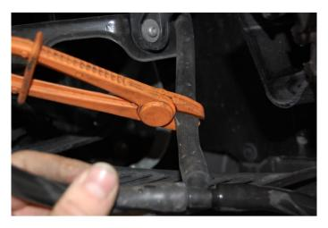
**Step 23:** Unclip the hose from each washer nozzle and lift the bumper aside.
