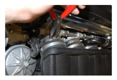
**Step 14:** Lift the manifold up in the front and remove the oil drain hose on the underside of the manifold. Lift the manifold out of the car.
