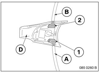
Connect the black 4-pin socket casing (1) on adapter cable **A** and the violet 4-pin socket casing (2) on connection cable **B** to switch **D**.
