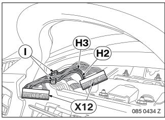
Disconnect plug **X12** from the light switch centre and open it.
