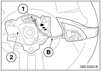
Connect the white 4-pin socket casing (1) on connection cable **B** to the steering column (2).
