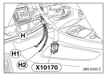
Disconnect plug **X10170** from the slip ring. Connect branches **H1** and **H2** to plug **X10170** as follows:
