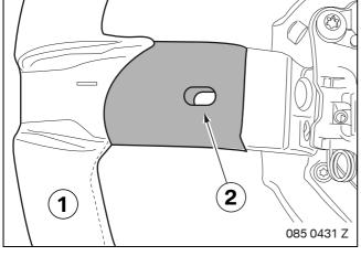
Cut the rigid foam off the steering wheel spoke (1) in area (2).
