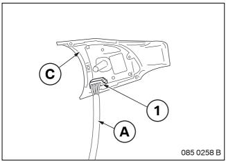
Connect the SW 4-pin socket casing (1) on adapter cable **A** to switch **C**.
