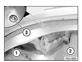
Release screws (1 and 2) and remove expansion rivet (3).
