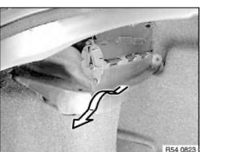
Feed out mounting towards rear top over spring strut cap.
