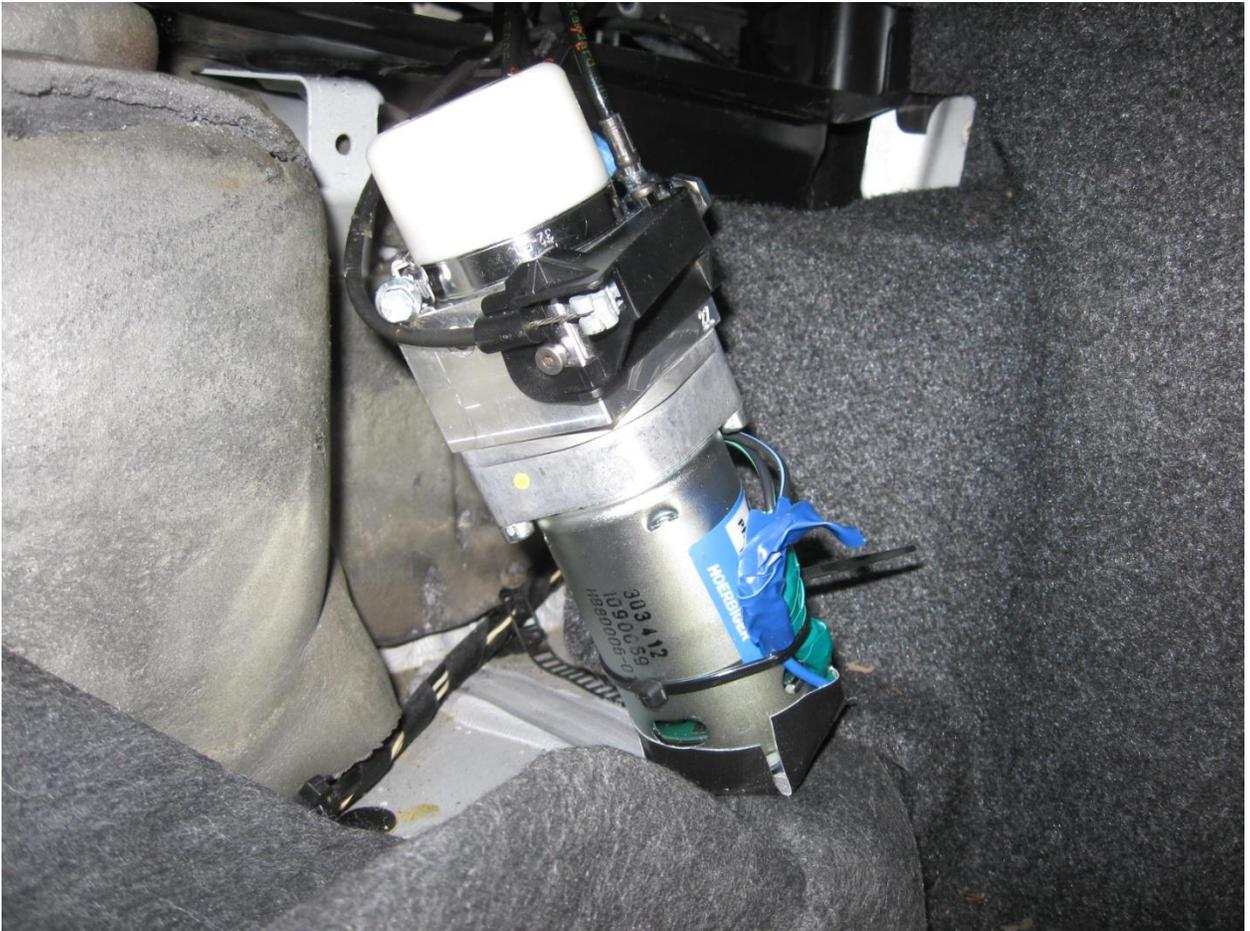
27. I also used some duct tape on the bottom of the motor to hold the connectors onto the motor terminals.
