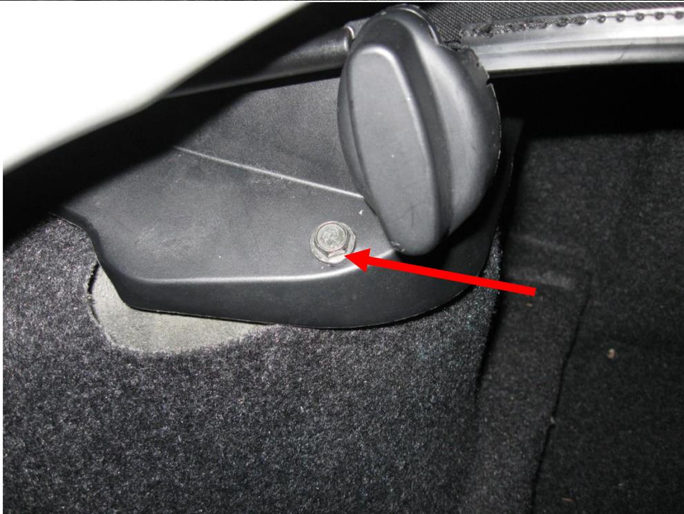
**Relocation of Soft Top Pump Assembly from the Drain Funnel to the Trunk
