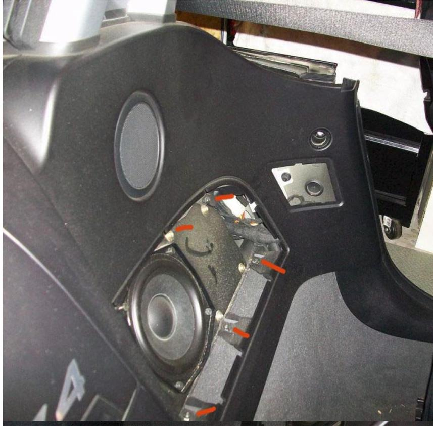
6. Pull the drive door weather strip out from underneath the seal at the top of the door pillar and pull it loose from the car body down far enough to free the edge of the rear plastic panel. Grasp the panel at the bottom outside corner and unsnap it from the car body.
