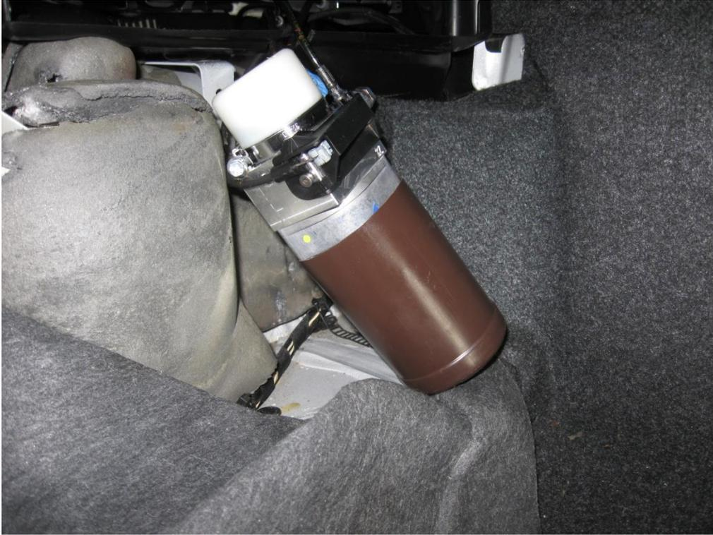
29. I installed a small cable clamp on the stud for the ground point on the side wall of the trunk to use as an anchor point for the motor.
