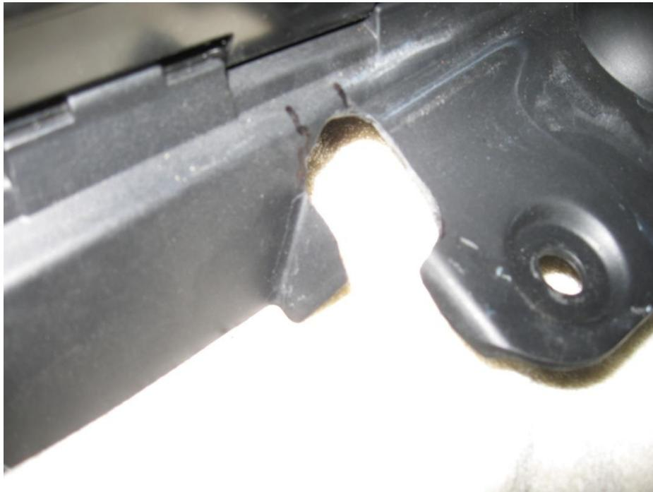
19. Route the hydraulic lines and the release cable through the slot in the side piece, then slide the tray support piece into position and fasten it place with the forward and rear bolts. **Don't put the plastic rivet back yet.**
