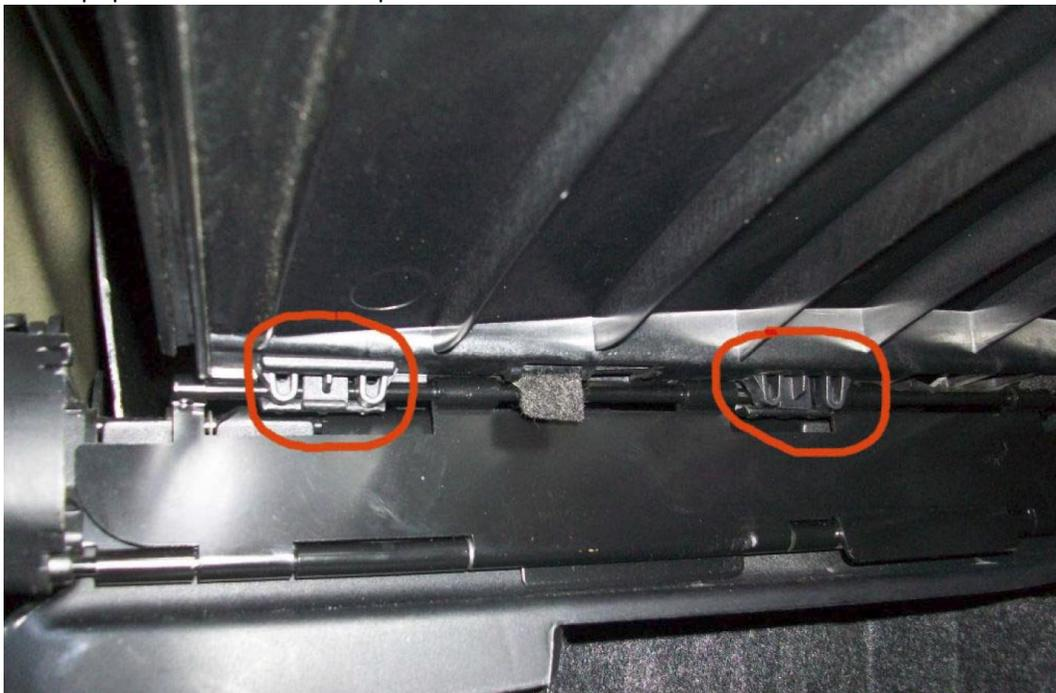
4. Remove the driver side tray holder. There's a bolt up underneath the front of it and one on the driver side shock tower. There's also one of the dreaded plastic push rivets on top. Grab the
