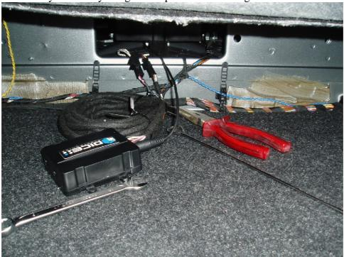
6: Hopefully it works! Follow the instructions in the user manual. Once I was confident it worked, I fed the docking cable through from the cockpit into the boot and then pulled it through the centre compartment and reconnected it to the DICE module
