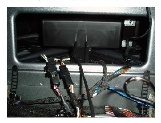
5: Time now to test it, so connect the docking cable to the DICE module then reconnect your battery. Plug in the ipod to the docking cable
