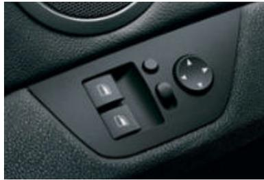
■ **Electric window lifts** incl. comfort control also controlled by the key by pressing and holding the central locking button on the key when locking the vehicle, open windows automatically close.
