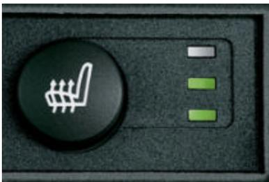
□ **Seat heating** for driver and front passenger ensures a pleasantly warm seat surface within minutes (three settings) (standard on Z4 3.0si<sup>1</sup>).
