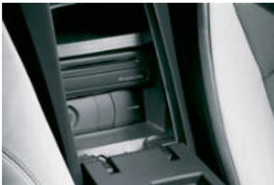
□ **CD changer, incl. MP3 decoder**, integrated into the storage compartment. The CD changer can hold up to six CDs (picture shows CD drive in combination with navigation system).
