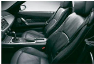
■ **Standard seat "Sport" for driver and front passenger**, deep moulded surface area, optimum lateral support in every driving situation provided by highly-contoured seat sides; wide range of settings even for taller people; individual adjustment for seat height and seat angle (shown here in Oregon leather Black).
