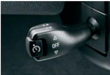
□ **Cruise control** lets you store and maintain a chosen speed (for speeds of 30 km/h and higher). Activated via the left hand side steering column switch. Deactivated by applying the brakes. After accelerating the set speed is automatically resumed.
