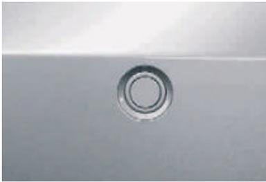
□ **Park Distance Control (PDC)** for the rear area; facilitates parking and manoeuvring in tight spaces. The distance between your car and any obstacle is indicated acoustically.
