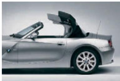
■ **Manual roof operation**, central lock for single-handed operation; thanks to the special folding mechanism no canopy or top lid is needed.
