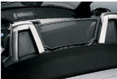
□ **Wind deflector** reduces irritating drafts and annoying isolated turbulence in the shoulder and neck region; consisting of two panes securely fitted into the rollbars and a frame-based net spanning between them. If the net is not required, it can be stored in a special storage rack in the luggage compartment.
