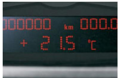
□ **On-board computer** provides data on average speed, average fuel consumption, range, time and outside temperature (standard on the Z4 2.5i, Z4 2.5si and Z4 3.0si<sup>1</sup>).
