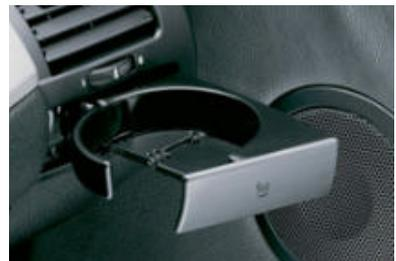
□ **Storage package** for even greater comfort inside; comprises storage nets at the back of the seats and the transmission tunnel as well as two touch-operated cup holders below the air vents on the left and right hand side.
