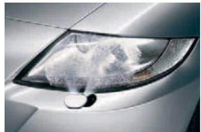
□ **Headlight washing system:** when the lights are on, the headlights are automatically cleaned in parallel with the windscreen whenever the right-hand steering column lever is activated.
