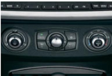
□ **Automatic air conditioning**, including AAR, rapidly provides the desired climatic conditions in the interior of the vehicle and maintains the selected temperature, including memory function for individual manual settings. The integrated Automatic Air Recirculation (AAR) ensures that pollutants in the air do not enter the vehicle above a certain concentration.
