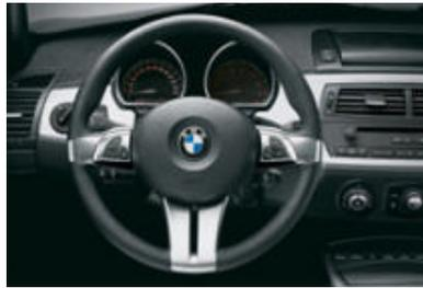
□ **Multifunction sports leather steering wheel**, control of radio and telephone (optional) via integrated buttons.
