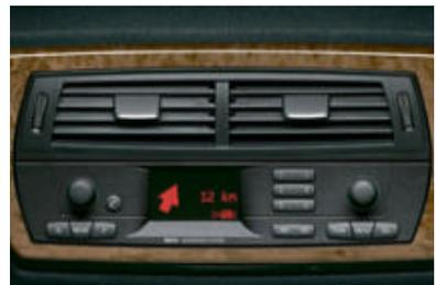
□ **Navigation system Business\*** incl. route planning with monochrome LC display integrated in the radio console (BMW Business Radio, without CD drive); traffic directions are provided exclusively by the voice computer and arrows on the display.
