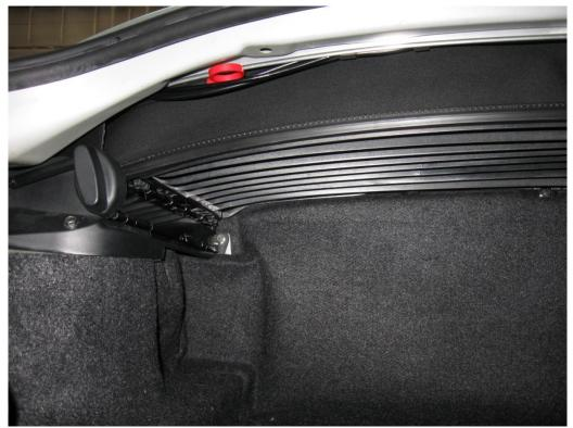
Then pinch and release the clips that are on each end of the floor. Note that there are locations for 3 each side but you'll likely only have two per side. They will pop up and lay on the side. Then unsnap the hinges by holding the floor with one hand and turning the floor lowering knob with the other. The hinges should pop loose from the floor piece.
