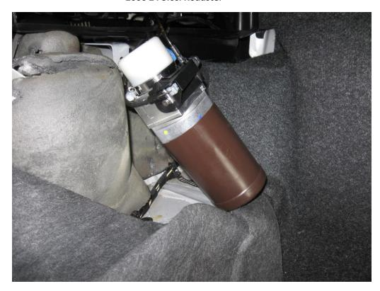
29. I installed a small cable clamp on the stud for the ground point on the side wall of the trunk to use as an anchor point for the motor.
