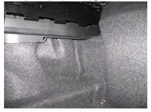
32. Reinstall the storage compartment tray, press the flap back onto it, and you're complete.
