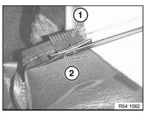
Secure rubber strap (1) and roofliner with <u>new</u> screw.
