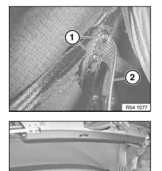
Secure tensioning strap and rubber strap (2) with new screws (1) to convertible top bow.
