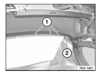
Attach screws (1) to convertible top bow. Attach screw (2) with rubber strap to convertible top bow.
