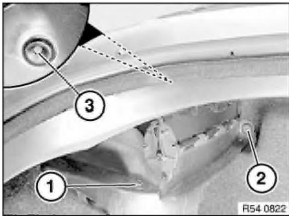
Release screws (1 and 2) and remove expansion rivet (3).
