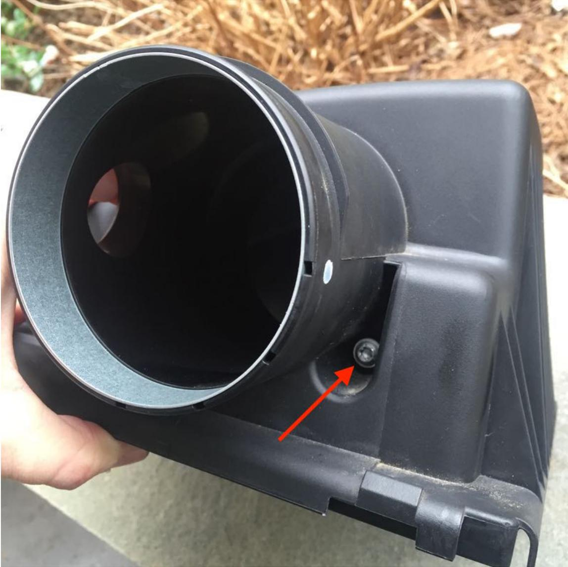
Next, pry around edges of the built-in filter in the top of the airbox to expose the inside.
