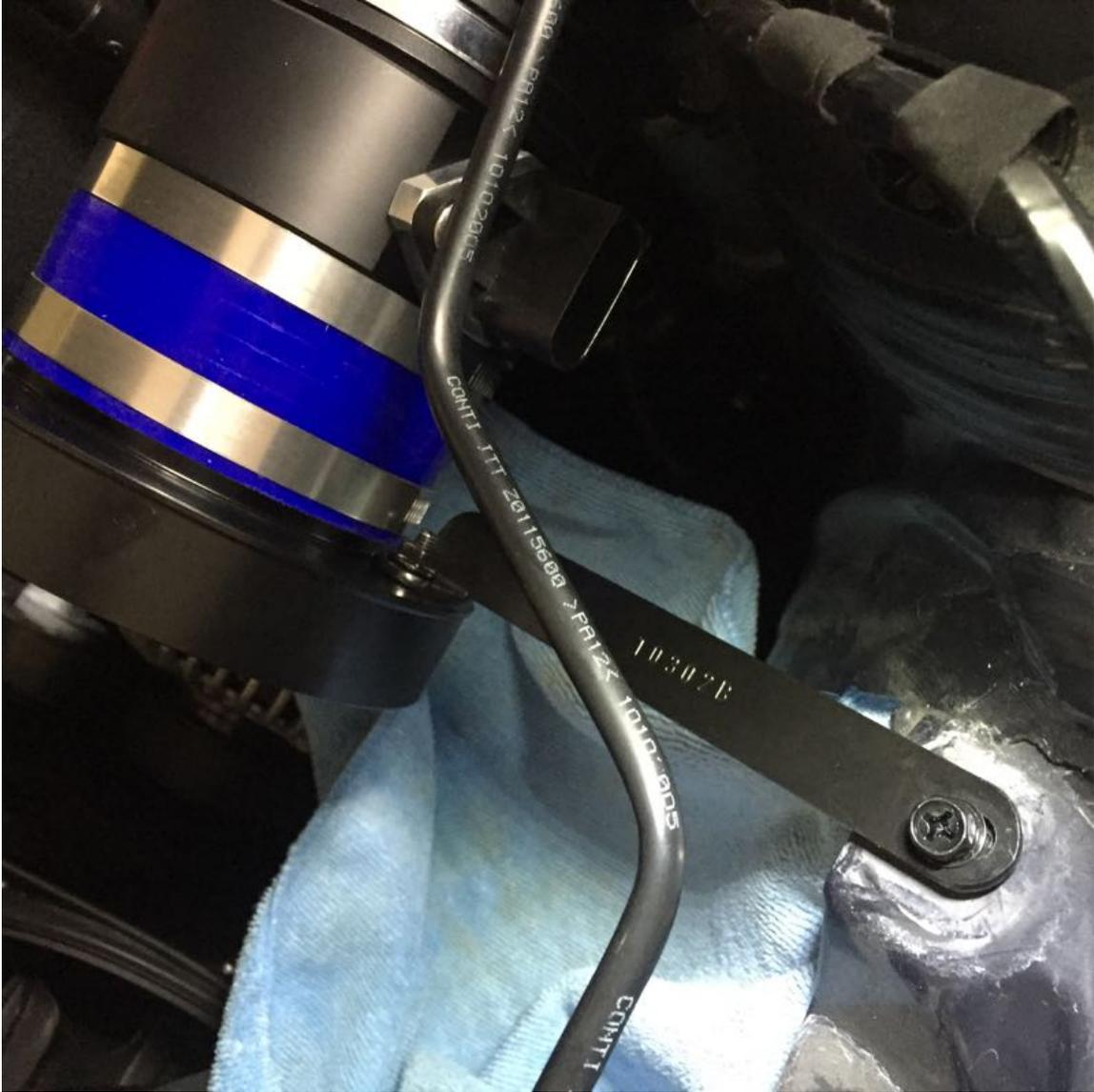
Reattach the MAF sensor connector, adjust the intake position, and tighten band clamps around the intake using the supplied allen wrench. Tighten band clamps around OEM inlet tubes.
