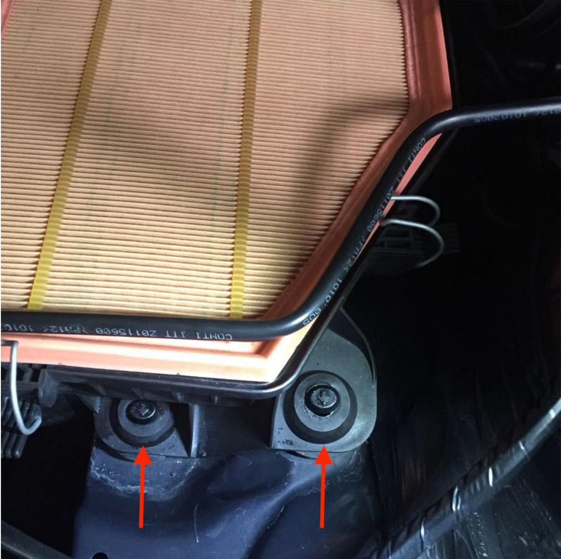
With airbox removed, you will now remove the upper connector to make room for the Gruppe-M intake support bracket.
