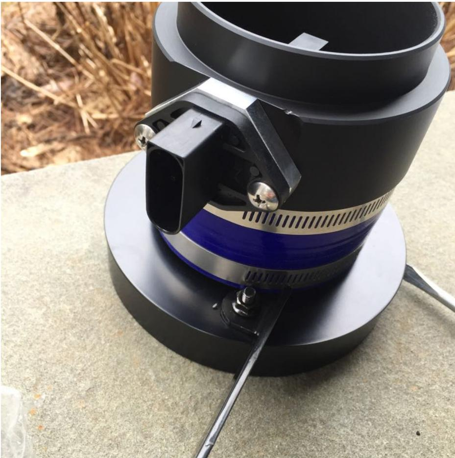
Attaching the support bracket requires holding a nut and washer under the small metal lip where the airbox was previously attached. This requires some finesse. A towel can be placed in this area to trap the nut and washer if they should fall. The bracket is held in place with bolt A. The carbon fiber intake is joined to the metal adapters by high quality band clamps. The intake should be placed roughly into position before mounting the support bracket.
