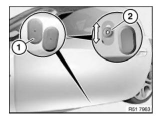
Adjustment by way of window guide rail: Open door and lever out rubber plug (1). Release nut (2) and move window guide rail. Tighten nut (2). Tightening torque 51 33 2AZ . Check adjustment, repeat procedure if necessary.
