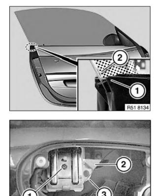
Sealing lip (1) of window cavity cover strip must not protrude over door window glass (2).
