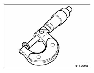
Measure removed adjustment plates.
