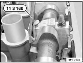
With cams pointing upwards, measure valve clearance with special tool 11 3 160 .
