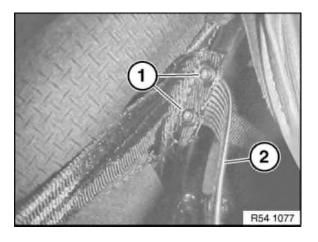
Secure tensioning strap and rubber strap (2) with new screws (1) to convertible top bow.
