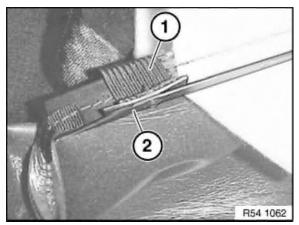
Secure rubber strap (1) and roofliner with <u>new</u> screw.
