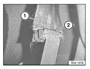
Secure rubber strap (2) to tensioning strap (1) with <a href="new screws">new screws</a>.
