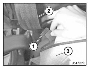
Feed rubber strap (1) from rear between convertible top cover (2) and roofliner (3) towards front.
