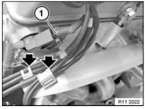
Disconnect plug connection (1) on sensor of exhaust camshaft.
