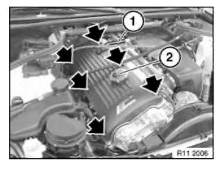
Remove hose (1) for engine vent.
