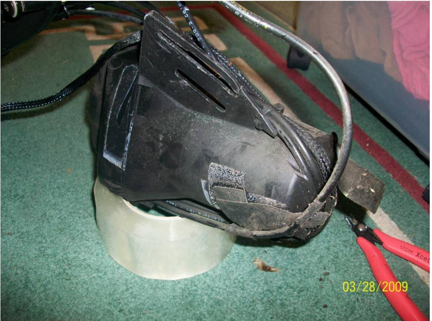
Remove the tape and tie-wraps from the cables and hoses.
