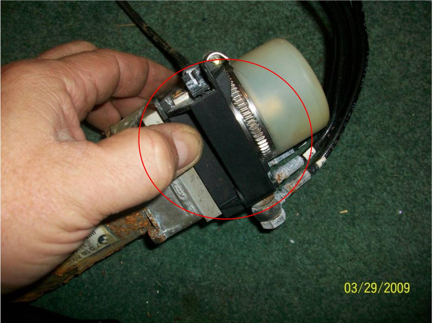
The Bowden Cable Assembly. Looking at the motor, the brass button on the bottom is the actual hydraulic by-pass plunger. This shifts the internal spool allowing oil to flow freely, without the motor driving it.
