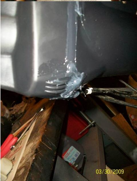
Now using the pictures I took, and remounted the unit to the frame making sure all the cables and hydraulic lines were running properly, additionally putting tie-wraps where needed.
