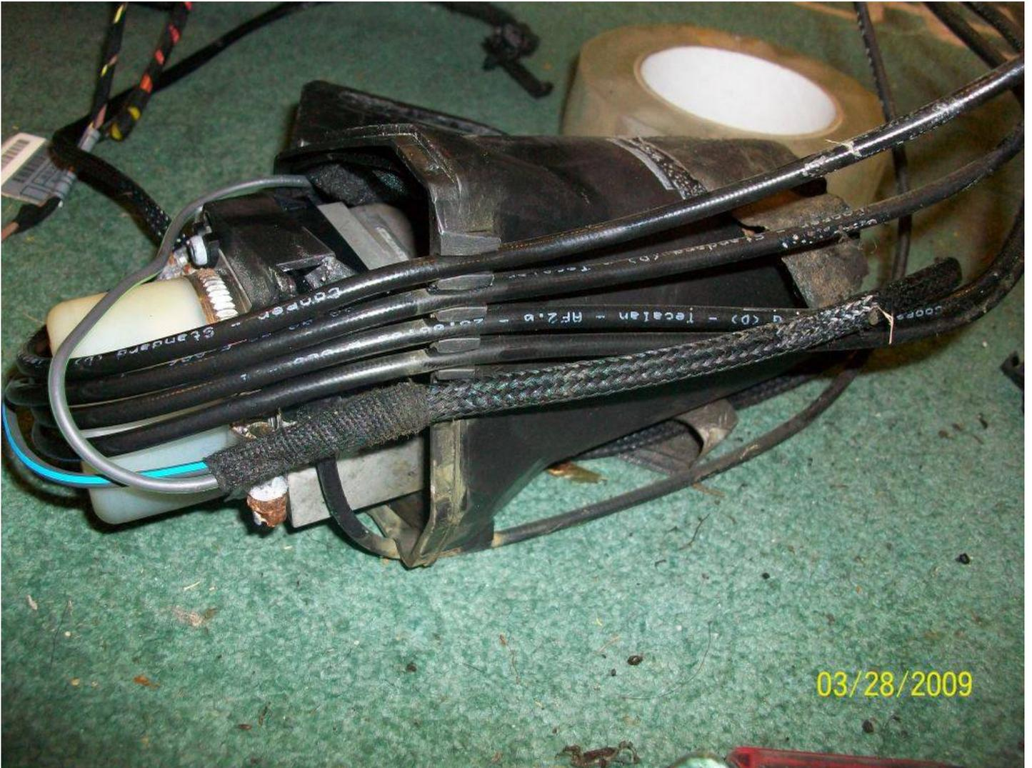
As extra insurance, before I pulled the motor out, I labeled the hydraulic lines. 3,4,5,6. and then after the motor was out of the housing, labeled the old housing the same way. Just to be sure.
