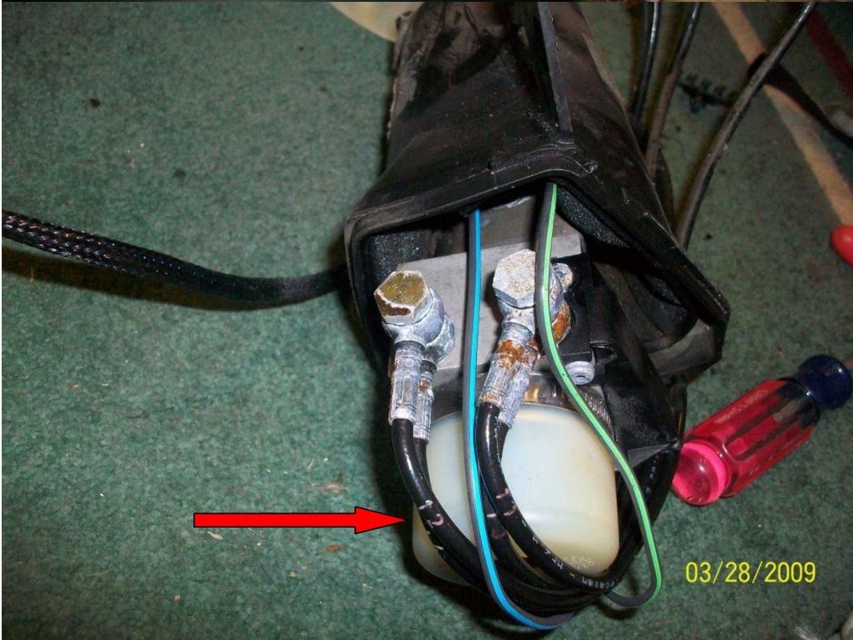
Remove the electrical connectors and clean them up. Use Q-Tips, Pipe Cleaners, whatever. I removed the boots and cleaned them up also. Carefully note which way the wires connect and what terminals they go on. If you put them on backward, the top will operate in reverse and you will have to remove the soft top and redo. 🚗
