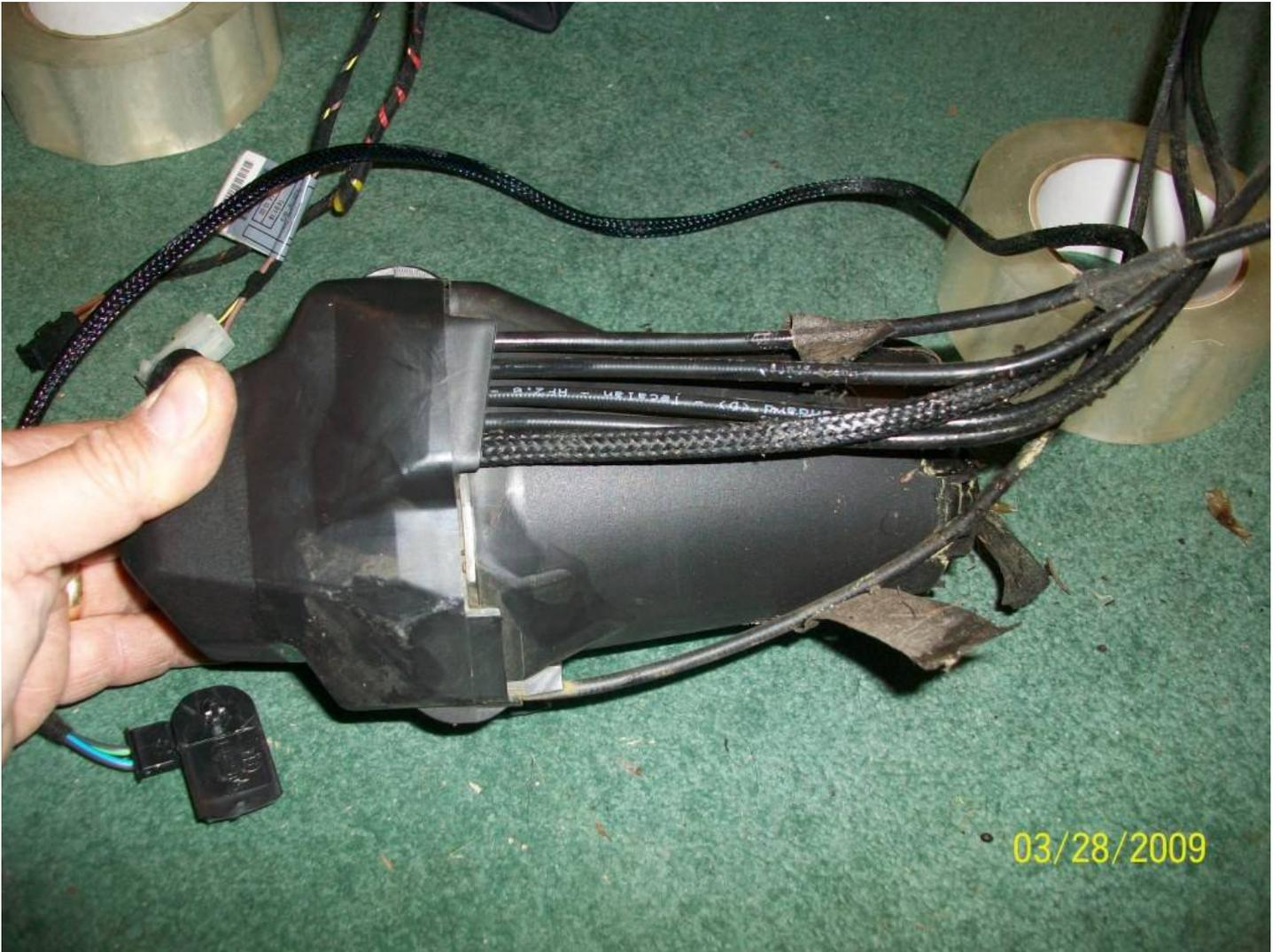
Housing cover removed. You can already see the corrosion.
