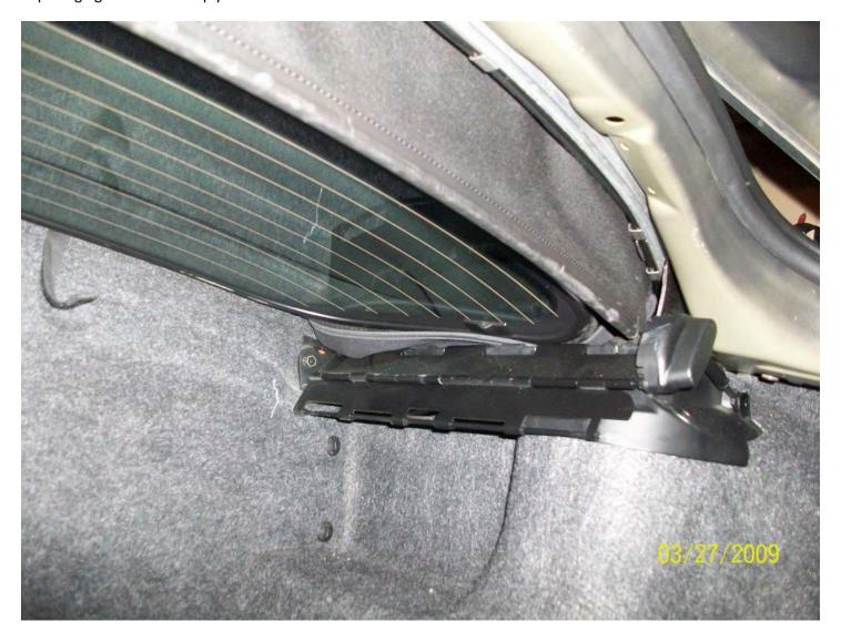
6. Now remove the weather stripping that attaches the top to the car. Only remove it from around the car body, NOT from the top itself. Don't try to remove it from the top or you will be buying a new top....
