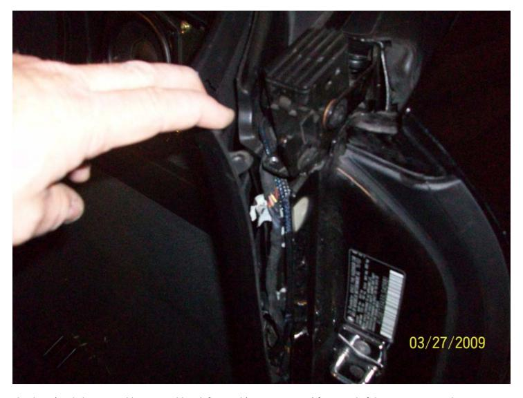
The driver's side has two cables. One cable is bifurcated (two connectors) for a total of three connectors. The passenger's side has just one cable and connector.
