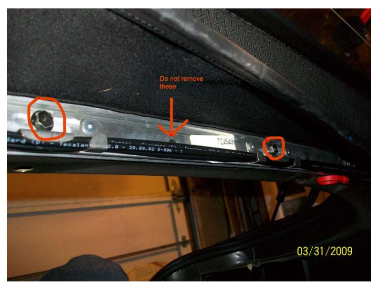
11. Now take your torx bits and go back inside of your car. Behind the vents grills you removed, was a round plastic cover, that I also had you remove. These are the lower mounting bolts. Now using a torx bit, loosen these lower mounting bolts on both sides. These two bolts do not have to be removed. It won't hurt, but is is not necessary, once you get the top out of the car and see the mounting hardware.
