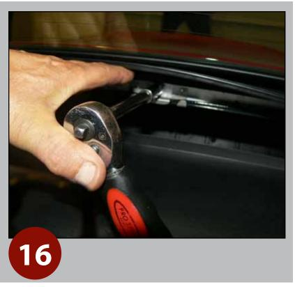
Cycle top to close position, detach rain flap and remove 10mm screws to free base bow.
