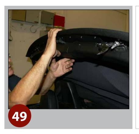
Install inner Torx screw first and then attach center cover to headliner panel.
