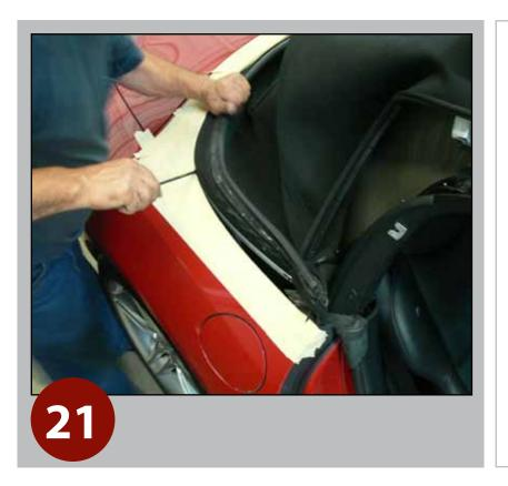
Carefully from either side, pry out base bow from top storage compartment.
