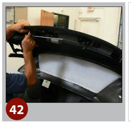
Install Torx screws across the header to secure top to frame.
