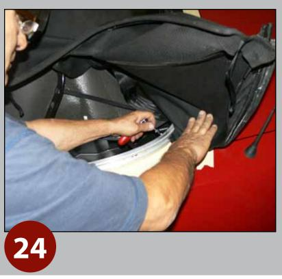
Continue to remove backside Torx screws to release top from base bow.
