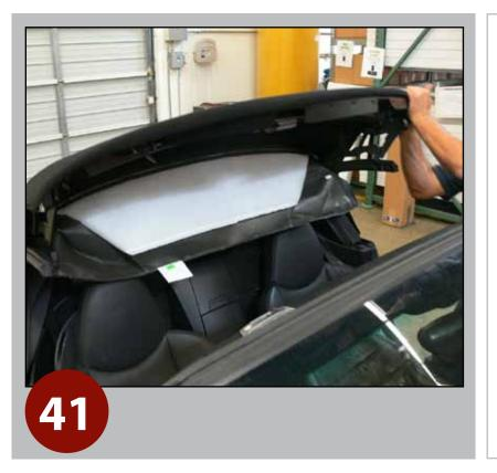
Install by fitting top's header (L/R) pocketed corners to top frame.
