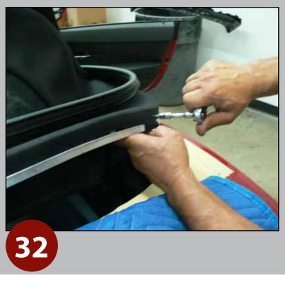
Install Torx screws (L/R), to support top to base bow.
