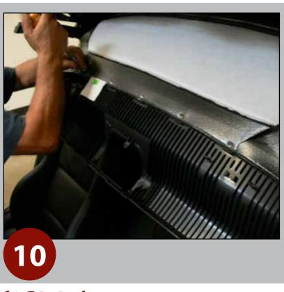
Remove Torx screws across the back edge of cover, to separate from headliner.
