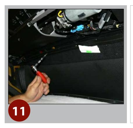
Remove Torx screws across the inside of header, to release headliner from frame.
