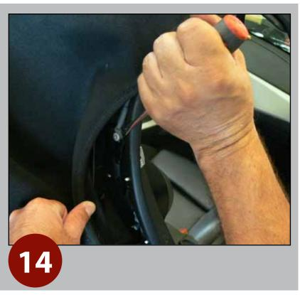
Drill or chisel rivet heads (L/R), to release the side tension cables from frame.
