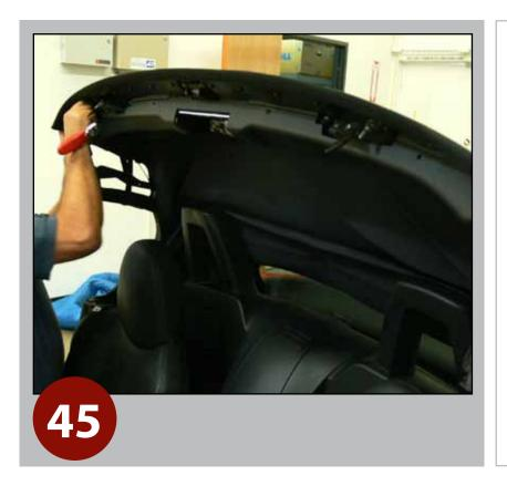
Position headliner panel across the frame header, and use Torx screws to secure.
