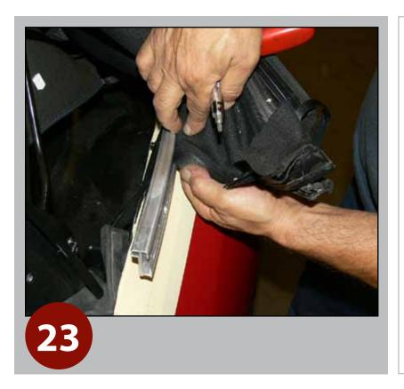
Start separating top from base bow, by force out plastic retainer from bow channel.
