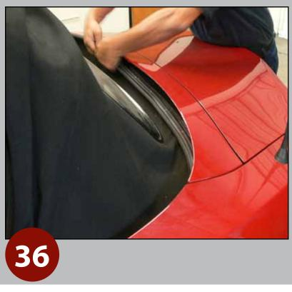
Cycle top to mid-open position, from either side connect base molding seal to vehicle.
