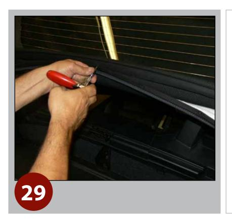
Install Torx screws to support headliner/top support flaps to rear bow.
