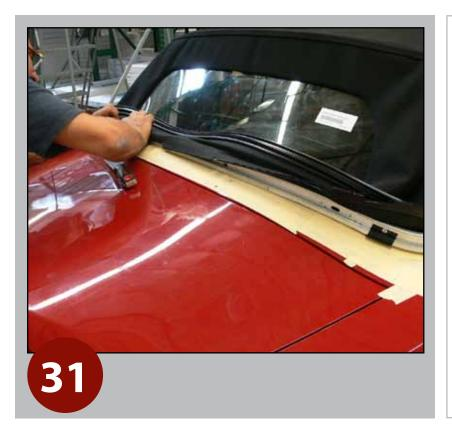
Position/center top's support flap to base bow, and insert retainer into bow's channel.
