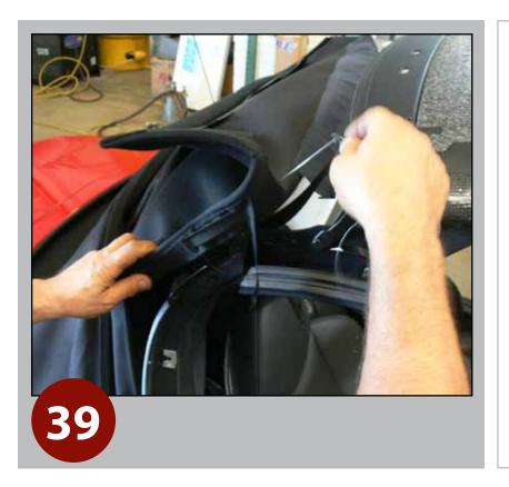
Cycle top to mid-open position, use hanger wire to insert (L/R) tension cables thru top.
