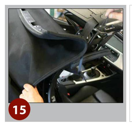
Carefully pull out (L/R) side tension cables from top's side pocketed sleeves.
