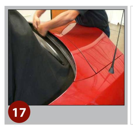
Cycle top to mid-open position, from either side unclip base molding seal from vehicle.
