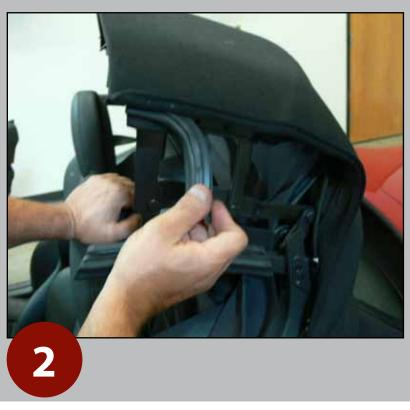
Carefully detach by forcing out (L/R) side (front) weather seals from top frame.
