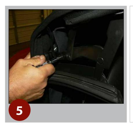
Remove Torx screws (L/R), to release top side support straps from frame.
