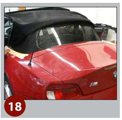
Use 2" tape all around the top storage edge, to protect paint from lifting out base bow.
