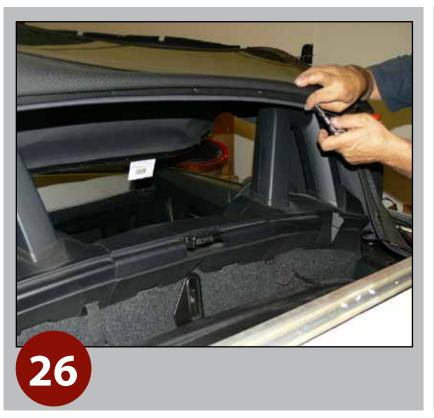
Flip top window forward; remove bow Torx screws to release top/ headliner from frame.
