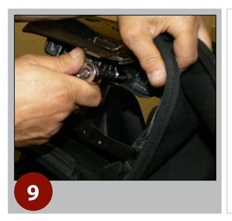
Remove side Torx screws (L/R), to release the headliner front cover from frame.
