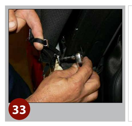
Install Torx screws (L/R), to attach top's quarter support straps to base bow.
