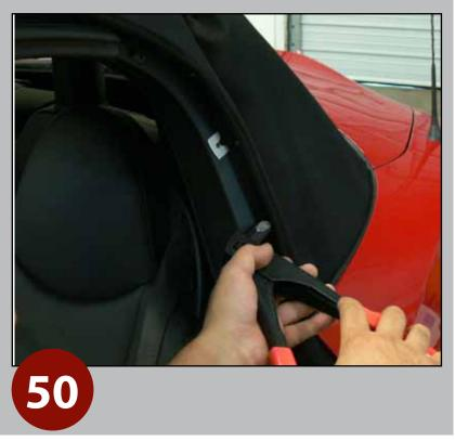
Cycle top to close position, align (L/R) top quarters to frame and use rivets to secure.
