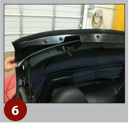
Detach the front edge of soft top from frame header, to continue removal.
