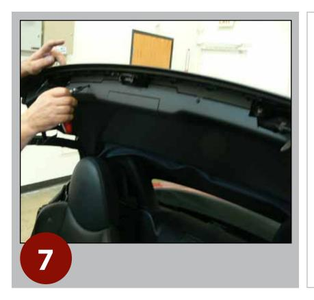
Remove Torx screws across the headliner panel, to release it from the frame.
