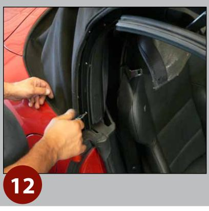
Detach (L/R) quarter seals and remove Torx screws to release seal brackets from frame.
