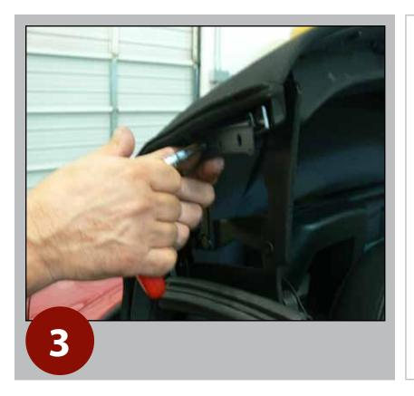
Remove Torx screws (L/R) to release weather seal brackets from top frame.
