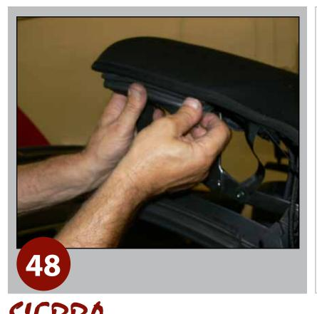
Install (L/R) side (front) weather seals onto frame.
