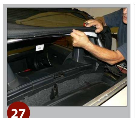
Detach top/headliner support flap from rear bow and remove complete top from frame.
