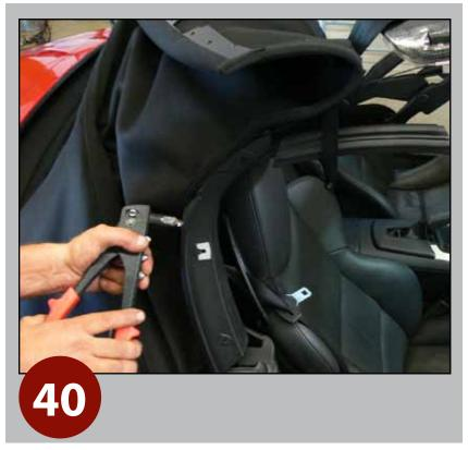
Use 4mm rivets to secure (L/R) tension cables to top frame.
