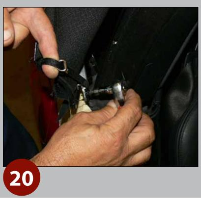
Remove inner Torx screws (L/R), to release top's quarter straps from base bow.
