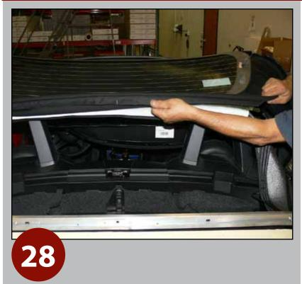
Apply contact cement to rear bow; locate/mark center, attach support flap to rear bow.
