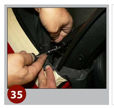
Install Torx screws (L/R), to attach top's quarter straps (with O-ring) to frame.
