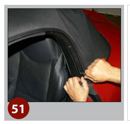
Install Torx screws to secure (L/R) quarter weather seal brackets to frame.
