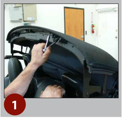
Cycle top to mid-open position, remove Torx screws across header to release top.
