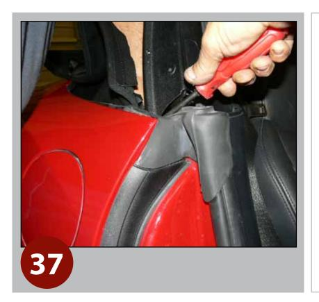
Use a flat-head screwdriver to help assist, tucking top's quarters into compartment.
