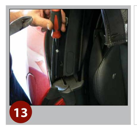
Drill or chisel rivet heads (L/R), to release top quarter retainer attachments from frame.
