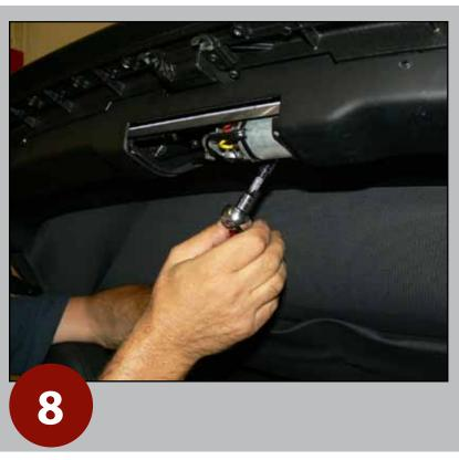
Detach center cover and remove the inner Torx screw, to release cover from frame.
