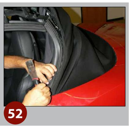
Cycle top to mid-open position, install (L/R) quarter weather seals to frame.
