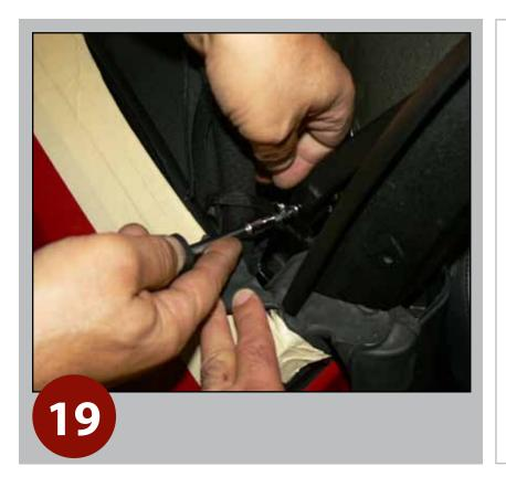
Remove Torx screws (L/R), to release top's quarter straps (with O-ring) from frame.
