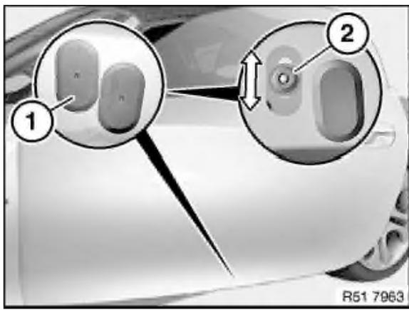
Adjustment by way of window guide rail:
