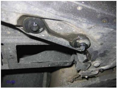
Make sure to unclip the ABS/DSC sensor that is clipped onto the splash thingy:
