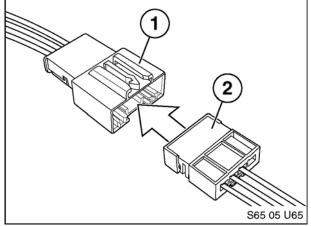
6. Insert 3 rectangular pins from iPod harness (1) into radio harness (2) as follows:
