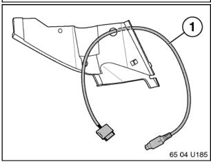
12. Insert iPod cable (1) through hole in glove box as indicated.
