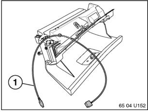
11. Insert iPod cable (1) through hole in glovebox as indicated.
