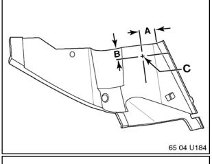
11. Locate and drill 5/8" (16mm) hole in glove box.
