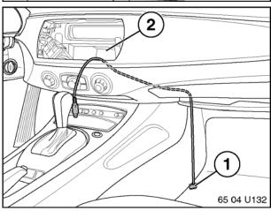
11. Insert iPod cable (1) through hole in glovebox as indicated and route through radio cavity (2). A wire fish will be beneficial for this step.
