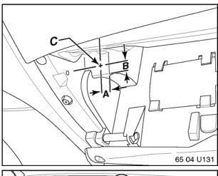
10. Locate and drill 5/8" (16mm) hole in glove box upper right panel.
