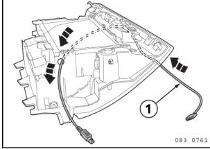
11. Insert iPod cable (1) through hole in glovebox as indicated.
