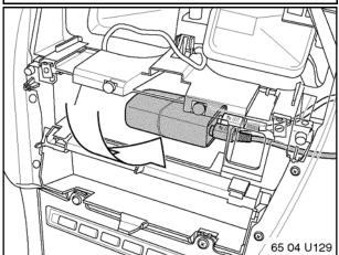
Caution: Check for bent pins on adapter cables before attaching to iPod module. If pins are damaged carefully bend them back into position with a small screwdriver.
