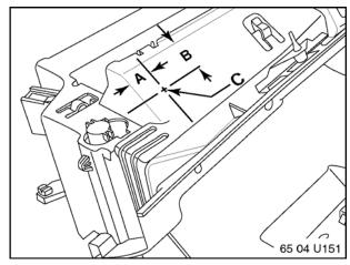
10. Locate and drill 5/8" (16mm) hole in glove box.
